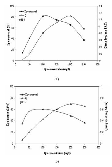
Fig. 3. Effect of initial dye concentration on dye removal efficiency and Q for: (a) PAC, (b) Alum
