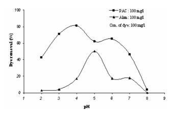
Fig. 1. Effect of pH on the removal of AR398 dye with PAC and Alum
